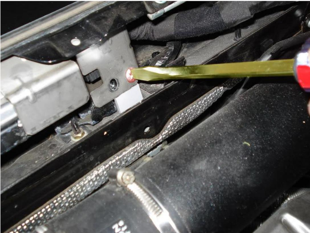
9. Work the Ecu out of the slot by sliding towards the driver side. NOTICE that i bent the cradle holders (yellow to red) right side to ease it out. you can do this IF YOU WANT .. since its strong enough to go back into place when i install the ECU it doesnt matter to me.
