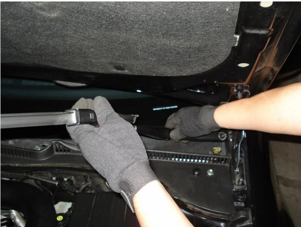
3. I didnt get a pic of removing the rain tray but its pretty easy.. just remove the liner and pull up and out on the rain tray and it will seperate. This pic is of the missing rain tray (yellow) and the exposed ECU (red)
