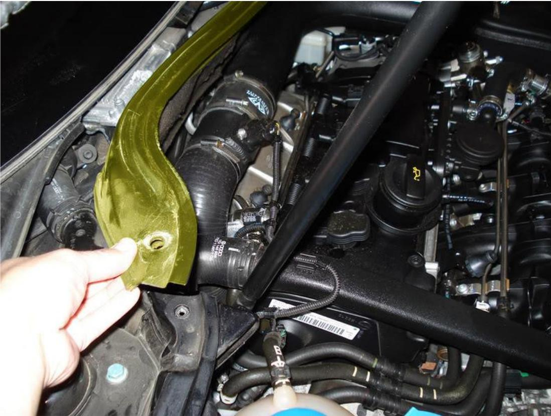
6. This is the driver side of the guard (yellow) that has the screw (red) near the battery
