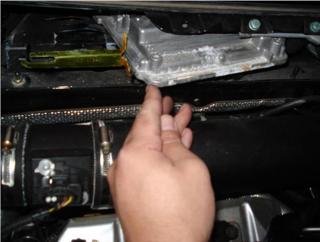
10. The ECU is out! but wait i have two thick cables still attached 😬
