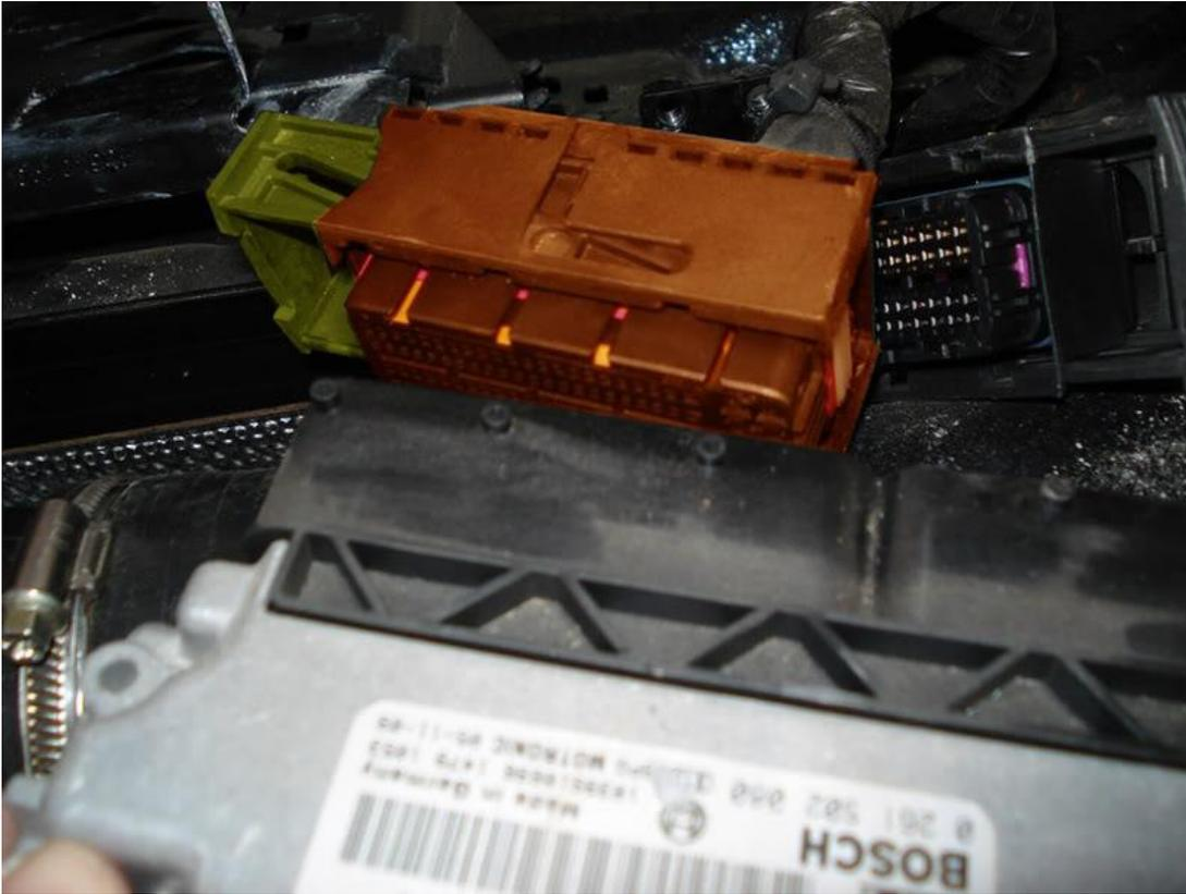
14. Remove ECU completely from the car!
