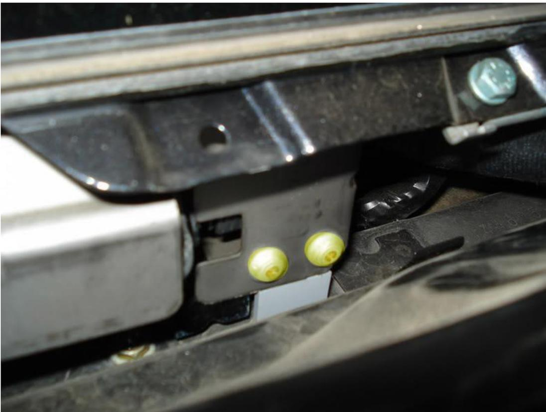
5. Now remove the screws to the removable guard (yellow).. one on the far left near the coolant ball and the right one is near the battery.
