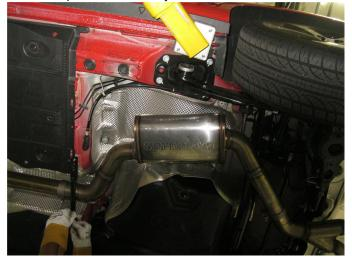
**Step 3.** Next attach the Muffler Assemby to the Inlet Pipe using the supplied 3.00" clamp and by fitting the hangers into the rubber insulators. Use the supplied Rubber Insulator for the welded hanger rearward of the muffler if applicable.
