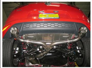
**Step 4.** Next attach the Y-Pipe Assemby to the Muffler Assembly using the supplied 3.00" clamp. Install the two Tail Pipe Assemblies in a similar fashion using the supplied 2.50" clamps. Locate the welded hangers to the rubber insulators.
