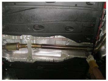
**Step 2.** Begin installing the new system by inserting the inlet of the Inlet Pipe into the OEM clamp at the catalytic converter. Leave clamp loose for final adjustment.
