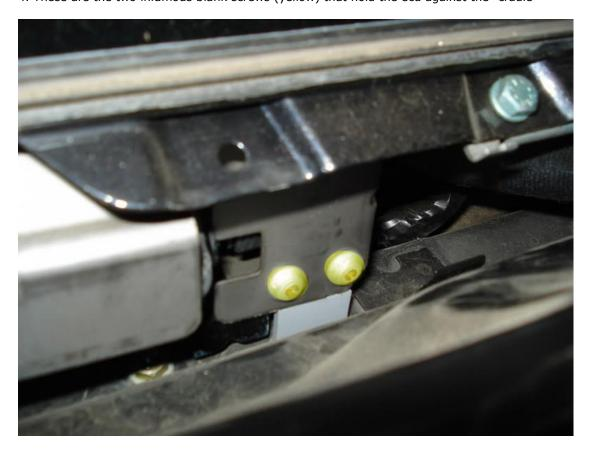
5. Now remove to screws to the removable guard (yellow).. ones on the far left near the coolant ball and the right one is near the battery.
