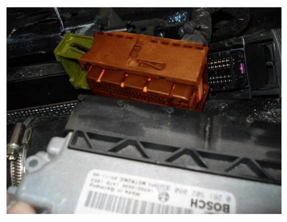
14. Remove ECU completely from the car!
