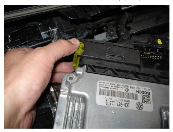
12. The drawer (yellow) is completely pulled to its fullest position
