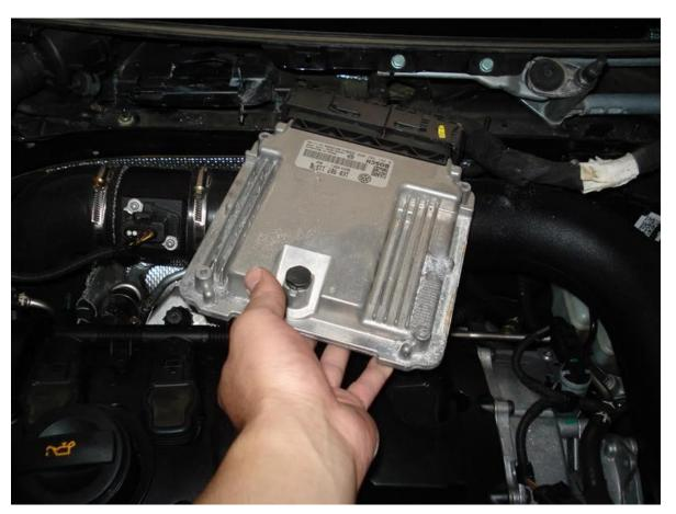
11. The two big cables connected to the ECU are secured by drawer clips (yellow). just pull outward
