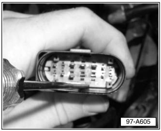
Open secondary lock for 14 pin connector (slide past lock tabs using small screw driver).
