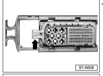
Remove purple secondary lock for 8 pin connector block (arrow).
