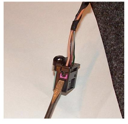
To remove the wires you must first remove the pink retaining clip.
