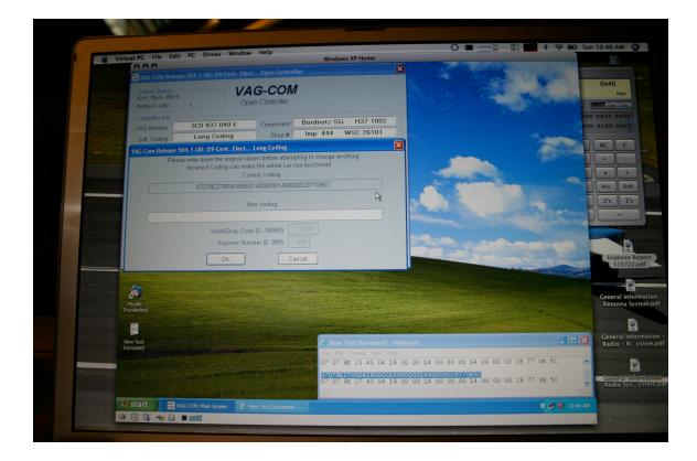
Now, comes the difficult part. You need to re-code module 9 to get the turn signals to blink amber properly and the brake lights to go on properly.
