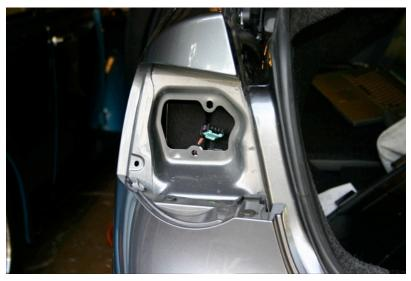
After removing the upper and lower 10mm nuts you can now pull out the taillight. You will have a hole in your car like this.
