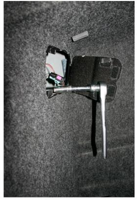
Using the 10mm ratchet and socket remove the upper and lower 10mm nuts.
