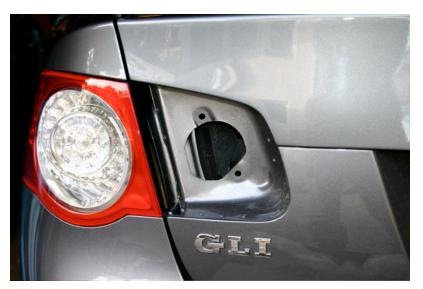
Here is what you will be left with after removing the trunk light. The same procedure applies for the passenger side.
