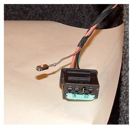
To remove a wire insert your "U" shaped tool into the slots above and below the main connector and push on it until the connector has slid out of the harness enough for you to pull it the rest of the way out.
