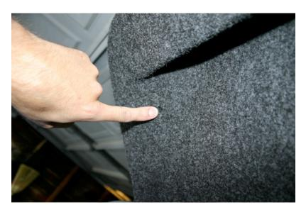
To remove the trunk lights locate the small hole in the trunk liner and insert a screwdriver to pull it loose.
