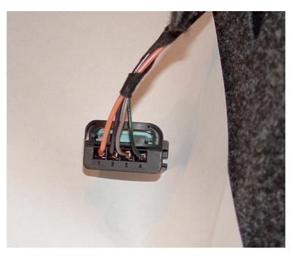
For the passenger side you need to remove PIN 4 and moved to PIN 3. PIN 3 will move to PIN 2 and the wire from PIN 2 will go to PIN 4,
