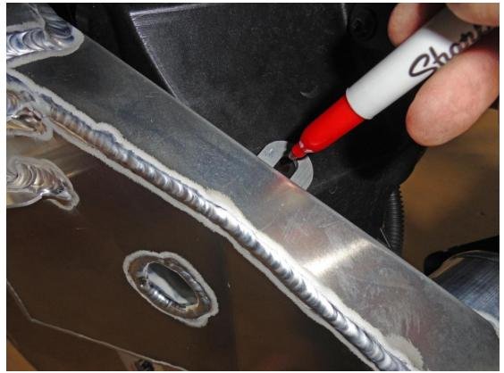
16. Drill a **shallow** 4mm hole in the centre of each of your marks, and if you wish use the screw to tap out its own thread while the core is removed. Then use the supplied penny washers with each of the screws, and affix the core to the car.
