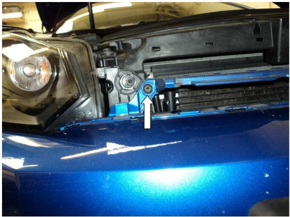
10. On both sides of the car pull down slightly and outwards on the corner of the bumper where it meets the wing. (READ THE NEXT 2 STEPS BEFORE DOING THIS AS YOU WILL SEE THERE ARE A FEW THINGS TO DO BEFORE THE BUMPER CAN BE REMOVED).
