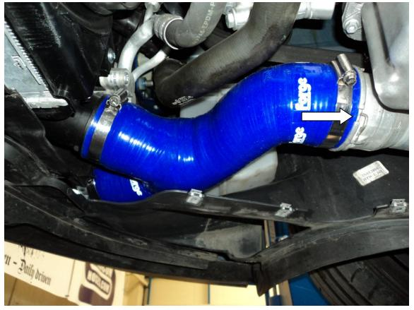
19. Under the car, remove the second clip from the front on both sides that used to retain the undertray. This is because the new silicon hoses are directly above them, and it will prevent you or anyone else accidentally putting a screw through the silicon hose.
