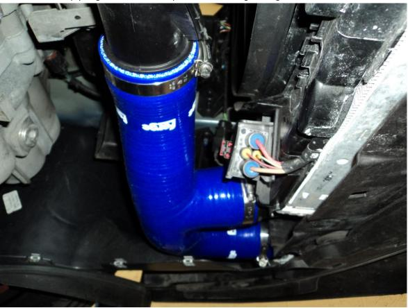
Use the provided bayonet coupler from step 7 to fit the hose to the turbo outlet. Once fitted, retighten the screws you loosened in step 16.
