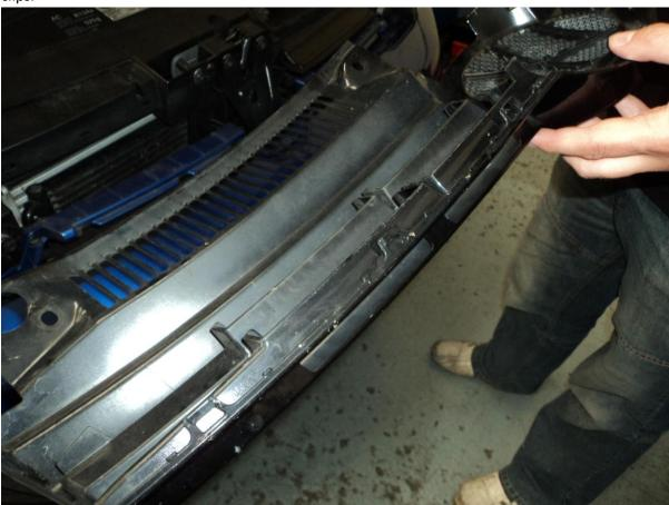
9. Undo the two T25 torx (one on each side of the bumper from where the grill was removed).
