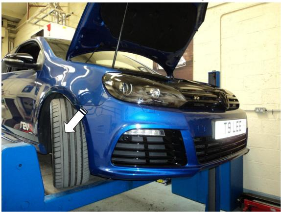
11. As you pull the bumper off you will have to remove some wiring. Firstly if you have parking sensors these will have to be unplugged (situated on the passenger side of the car), also on the driver side of the car you will need to remove the plug for the DRL's. Simply pull town on the tabs till you hear a click and then pull apart.
