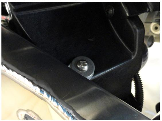
17. To enable easier fitment of the hose on the passenger side of the car, undo the two T30 screws holding the boost pipe to the lower edge of the block.
