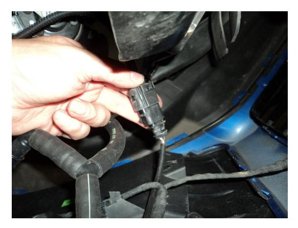
12. Next if you have headlight washers, these will need to be disconnected. To do this remove the "U" clip on the washer bottle pipe, situated on the driver side of the car and pull the connector from the pipe. You will need a bucket or bowl to catch the washer fluid.
