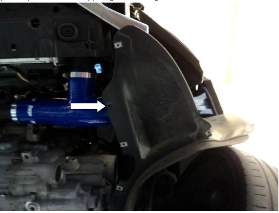
20. Lastly insert the air temp sensor removed in step 13 into the bracket on the front of the intercooler.
